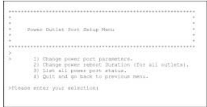
Figure 26 - Power Outlet Setup Menu (Terminal Screen)
